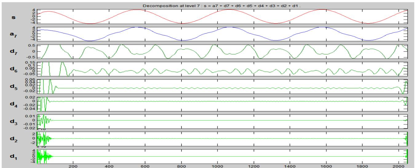
Fig. 7: Discrete Wavelet Transform of the phase current  $I_C$  under LIF condition
