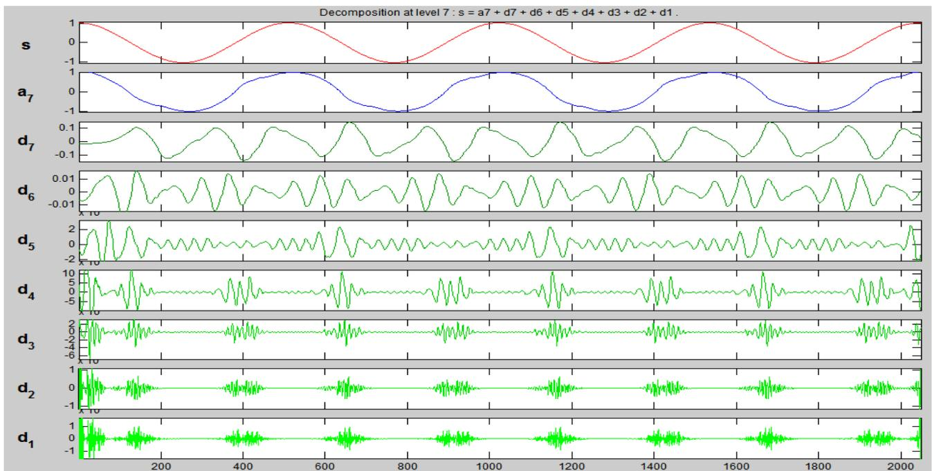
Fig. 6: Discrete Wavelet Transform of the phase current  $I_c$  under HIF condition
