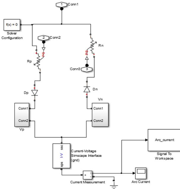
Fig. 5: HIF Simulink model
