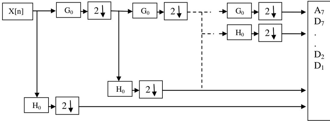
Fig. 1. Seven level wavelet filter bank
