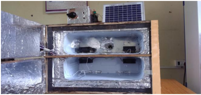
Figure 1: Designed Thermo-electric Heating & Cooling system.
