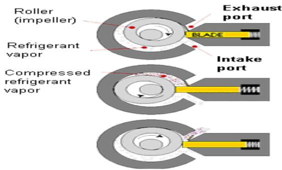
Figure 3: Rotary compressor
