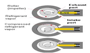
Figure 3: Rotary compressor
