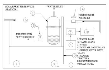
Figure 11: The Solar water service stations
