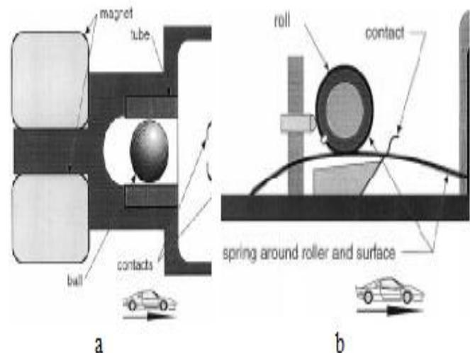
**Figure 1:** Two type of airbag activation sensors, a) tube sensor with damper, and b) spring-mass sensor [4].
