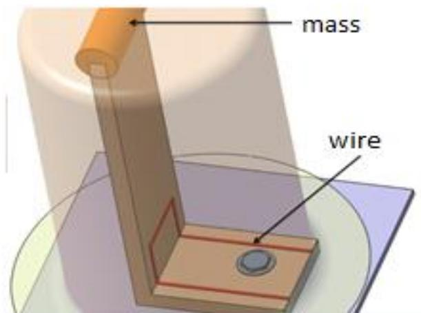
Figure 3: Designed mechanical sensor with an internal wire.
