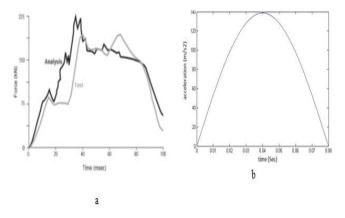
**Figure 4:** Variation of the force exerted on the car during the crash (a) from [7], simplified model of acceleration during the accident (b).
