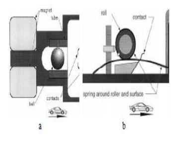
Figure 1: Two type of airbag activation sensors, a) tube sensor with damper, and b) spring-mass sensor [4].
