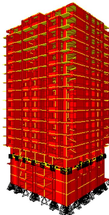
Fig. 6. Design model of the 17-story base isolated apartment building "Sevak"
